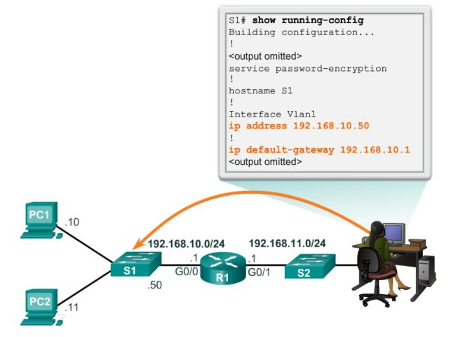
If the default gateway was not configured on S1, response packets from S1 would not be able to reach the administrator at 192.168.11.10. The administrator would not be able to manage the device remotely.
