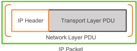
The network layer adds a header so packets can be routed through complex networks and reach their destination. In TCP/IP based networks, the network layer PDU is the IP packet.
