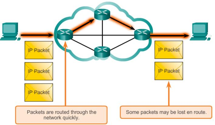
As an unreliable network layer protocol, IP does not guarantee that all sent packets will be received. Other protocols manage the process of tracking packets and ensuring their delivery.
