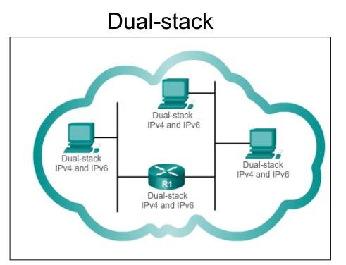
**Dual-stack:** Allows IPv4 and IPv6 to coexist on the same network. Devices run both IPv4 and IPv6 protocol stacks simultaneously.
