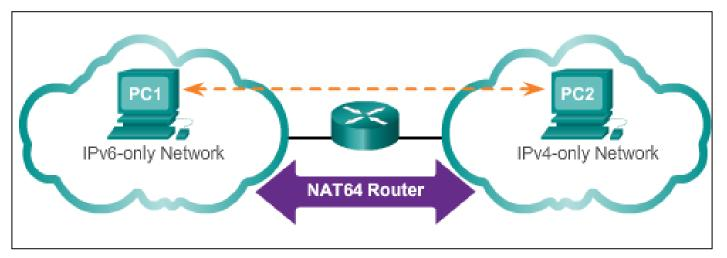
**Translation**: The Network Address Translation 64 (NAT64) allows IPv6-enabled devices to communicate with IPv4-enabled devices using a translation technique similar to NAT for IPv4. An IPv6 packet is translated to an IPv4 packet, and vice versa.
