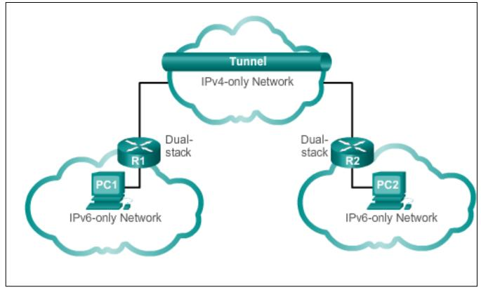
**Tunnelling**: A method of transporting an IPv6 packet over an IPv4 network. The IPv6 packet is encapsulated inside an IPv4 packet.
