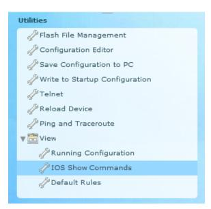
b. Select **show run** from the drop-down list and click **Show**. The router's running configuration is displayed in the content pane.
