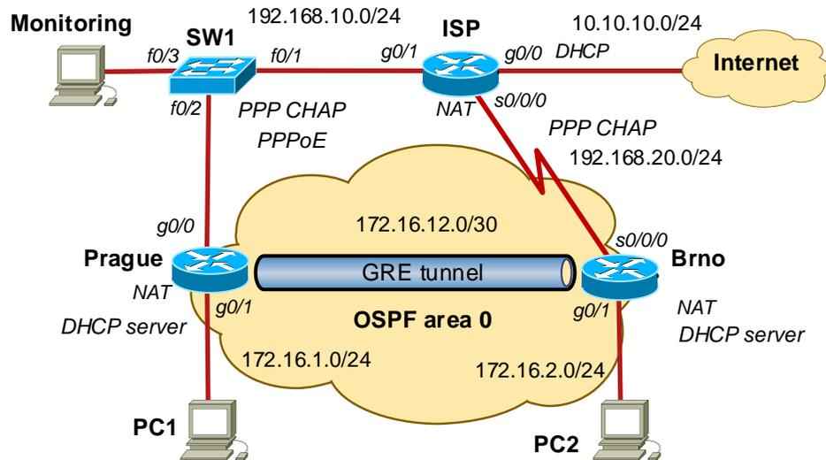
**Scenario Connecting Remote Branch Offices using VPN GRE Tunnel**
