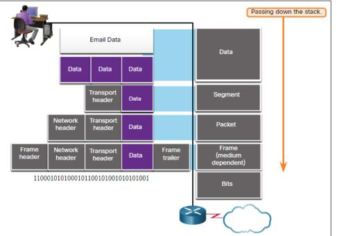
*Note*: If the Transport header is TCP, then it is a segment. If the Transport header is UDP then it is a datagram.
