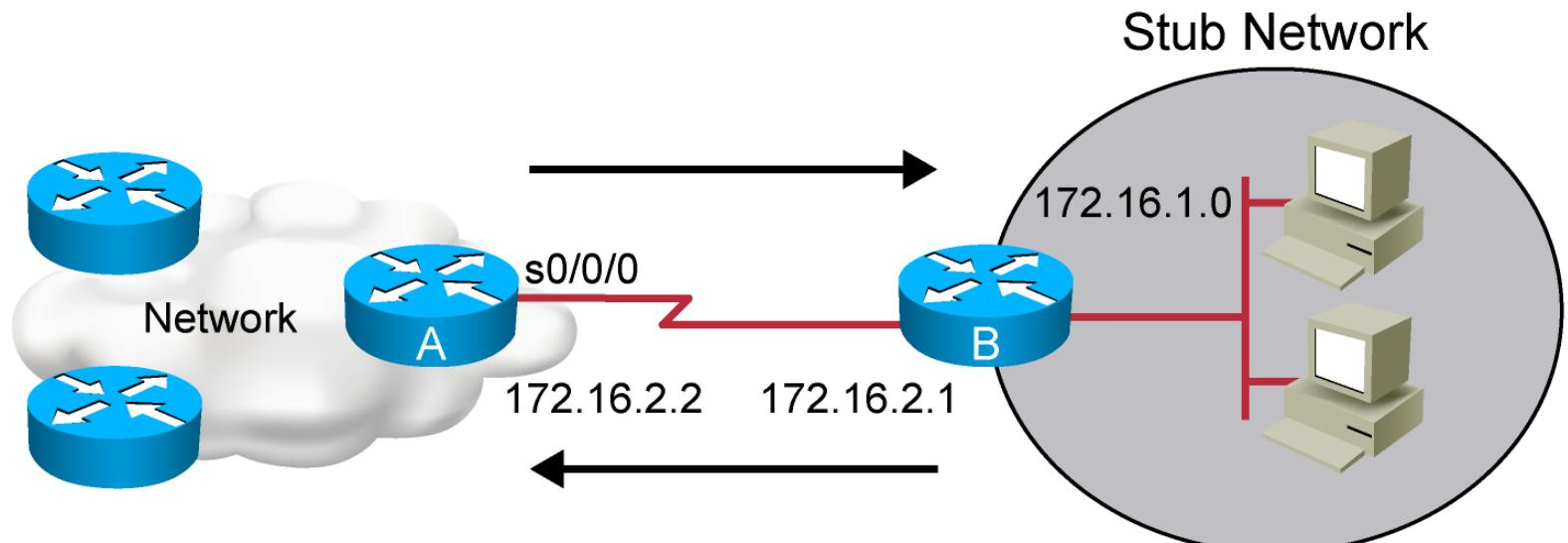
Configure unidirectional static routes to and from a stub network to allow communications to occur.
