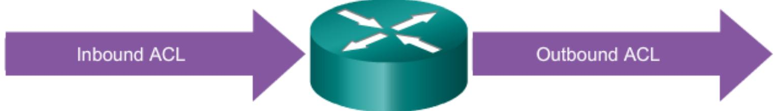
An inbound ACL filters packets coming into a specific interface and before they are routed to the outbound interface.
