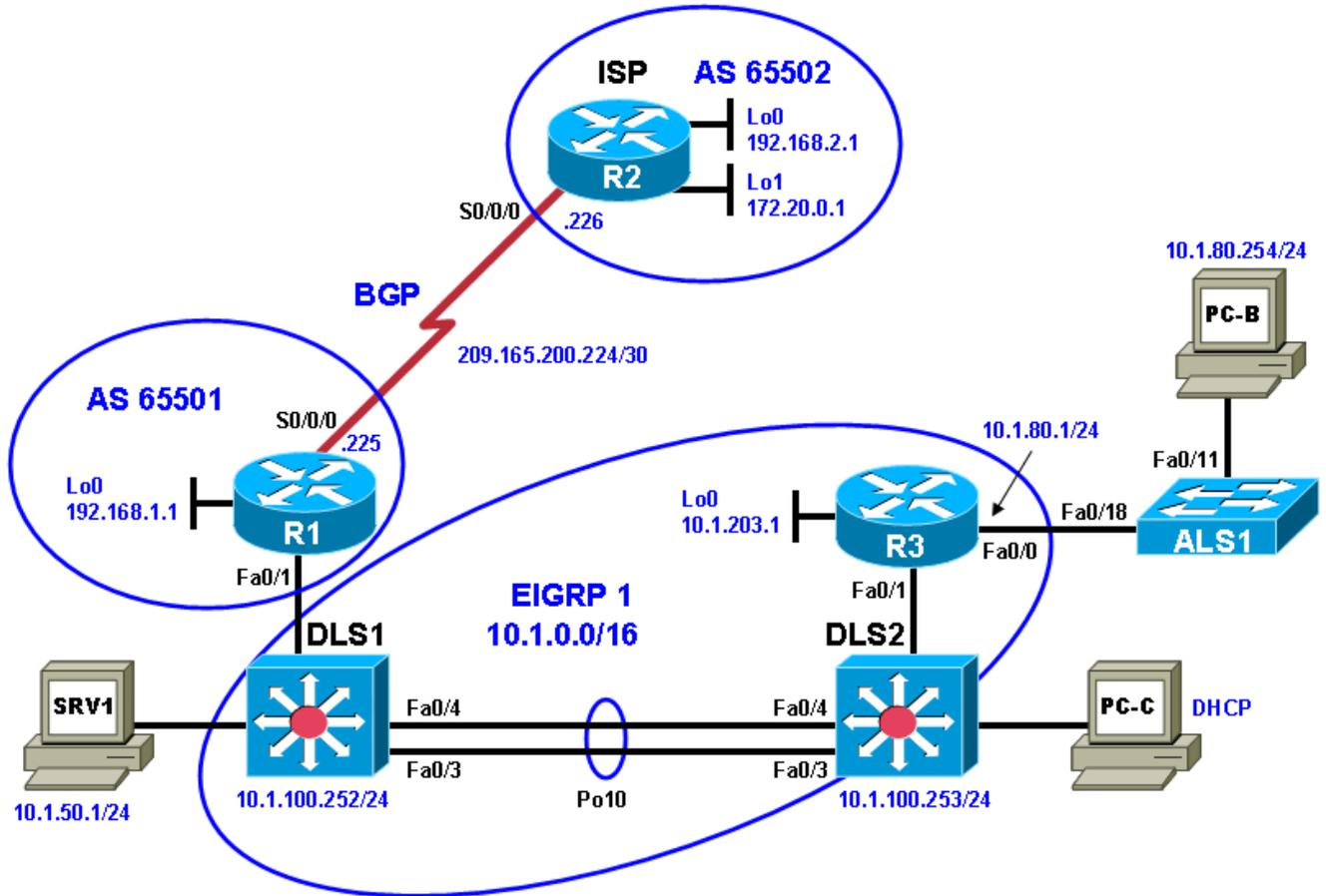
**Note:** The topology for this lab moves access switch ALS1 to R3 and disconnects it from switches DLS1 and DLS2. This allows a load to be placed on R3 using ALS1 and DLS2. PC-B is moved to switch ALS1 port Fa0/11. Performance testing is done using Cisco IOS commands on R3 and pings from PC-B. Even though ALS1 is no longer attached to DSL1 and DSL2, VLAN 10 still exists. The interfaces for port channel 1 on DLS1 and port channel 2 on DLS2 are temporarily shutdown.
